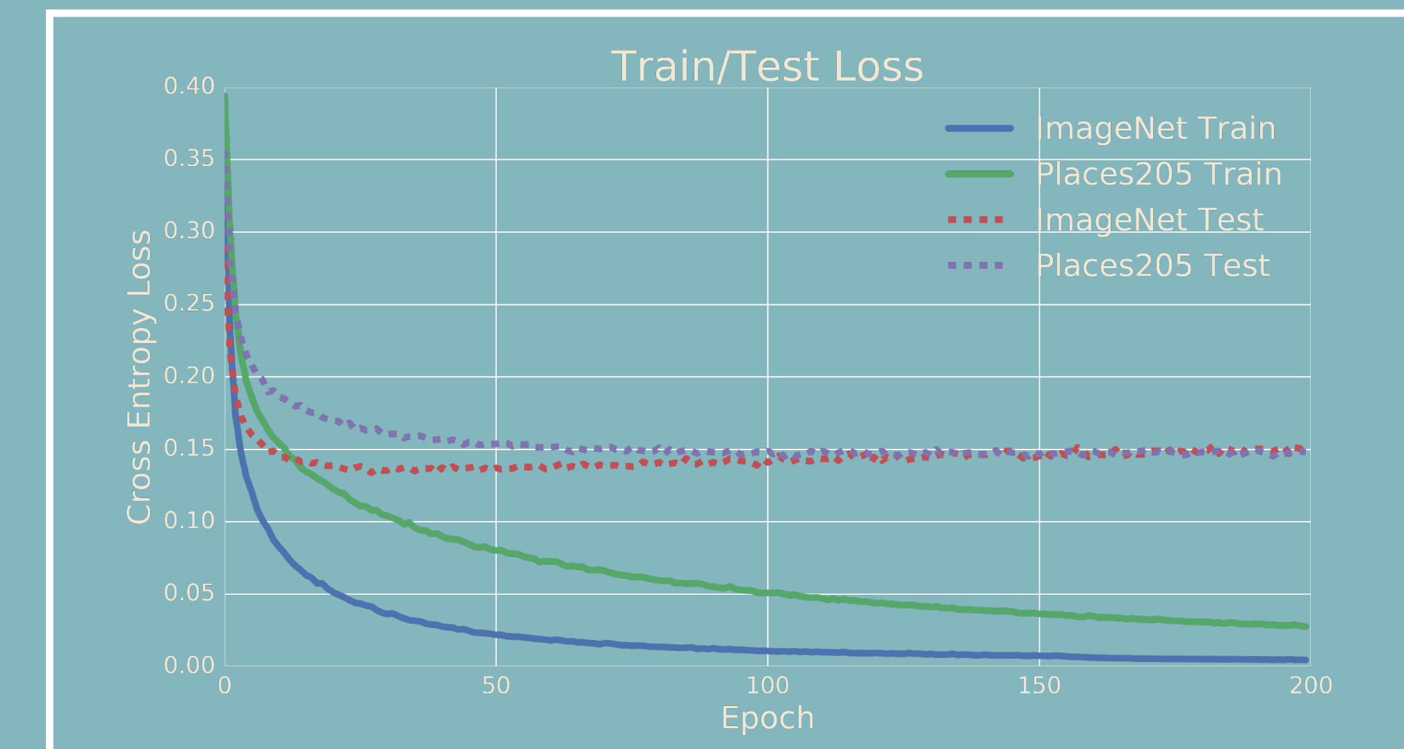
Fig. 4 (above): Supervised training on classification tasks results in nearly identical test loss at convergence. This indicates universality of distributed representations for later classification tasks.
